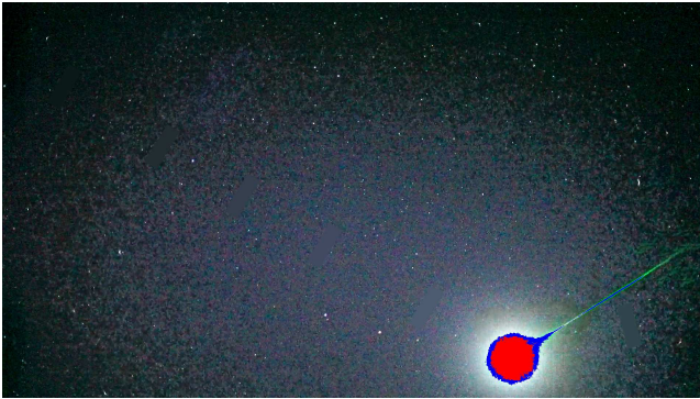
Figure 15 – Frame 01:50:59:22 of camera 2, terminal flash: 11076 overexposed pixels white = 11.4 arbitrary F stops and 6077 overexposed pixels green = 10.6 arbitrary F-stops. The terminal flash is much stronger in white than in green. This cannot be caused by a strong green overexposure, because than a green halo would be seen. But the halo around the terminal flash is white. Additionally, a bluish sky glow appears. (Also, the averaging of the code values inside the measurement fields can be seen.) The rectangular structures around and behind the meteor head are data compression artefacts caused by the camera.
